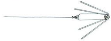
Fig. 22 A grapnel. When pulled through the water, the hooks collect pieces of plant.
