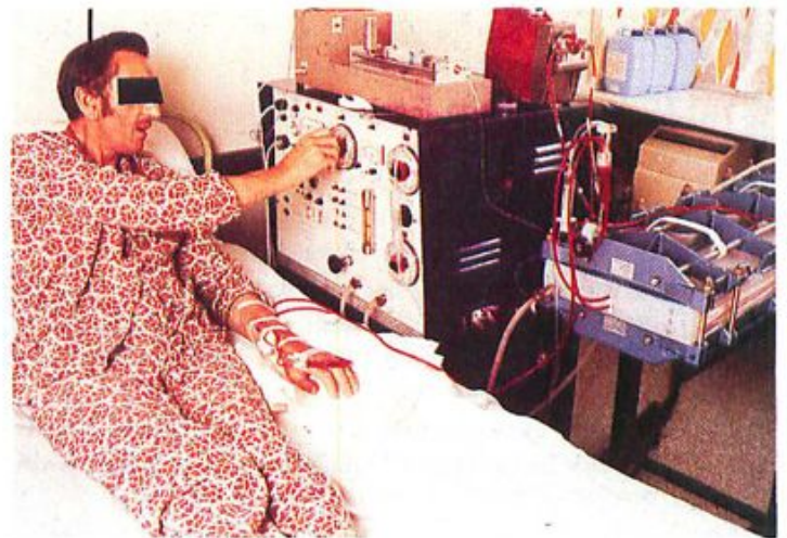
Fig. 8 Kidney dialysis machine. The patient's blood is sent by the pump (top right) to the dialyser (bottom right). The patient is adjusting the control box which regulates the temperature and concentration of the dialysing liquid.
